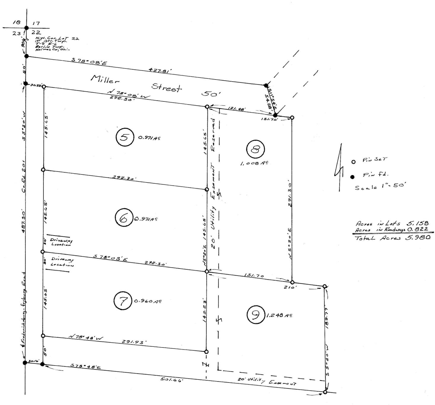
Central Water Will be Supplied by The Developer And Water Lines will be Laid Within The Utility Ensement as Shown.
