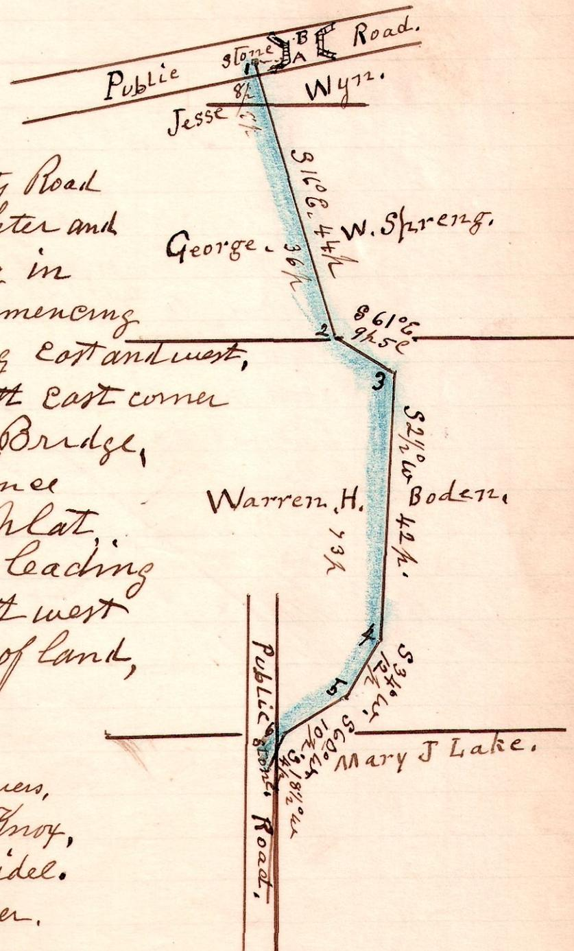
A Survey made of a County Road petitioned for by C. F. Wachter and others, the location being in Section 30, 3<sup>rd</sup> p. 18, Range 14, Commencing in the public road leading East and West, at a stone with witness, south east corner of west abutment to Iron Bridge, N 60° E. 1 perch + 22 links. Thence leading as indicated in plat, to end in public road leading North and South at North west corner of Mary J. Lakes lot of land, at a stone.
