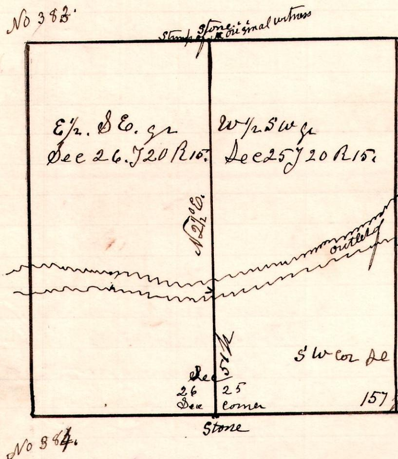
A Survey made for H. B. Curtis heirs, being the establishing of the line between the south west quarter of Section 25, and the south east quarter of Section 26, in Township Number 20 of Range Number 15.
